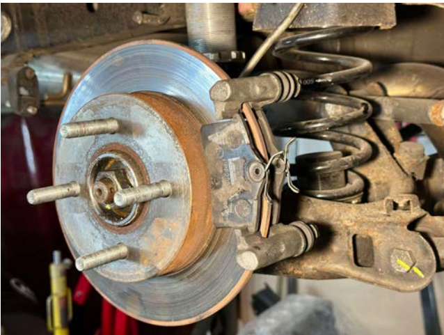
STEP 10 - INSTALL BRAKE HOSE (HOSE & PIPE IS NOT IN THE PICTURE AS MY RACE CAR USES A DIFFERENT SETUP - BUT IT WILL ATTACH TO THIS BRACKET ON THE CHASSIS WITH A CIRCLIP AND THE METAL LINE WILL SCREW INTO IT
