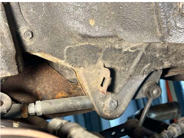
STEP 10 - INSTALL BRAKE HOSE (HOSE & PIPE IS NOT IN THE PICTURE AS MY RACE CAR USES A DIFFERENT SETUP - BUT IT WILL ATTACH TO THIS BRACKET ON THE CHASSIS WITH A CIRCLIP AND THE METAL LINE WILL SCREW INTO IT
