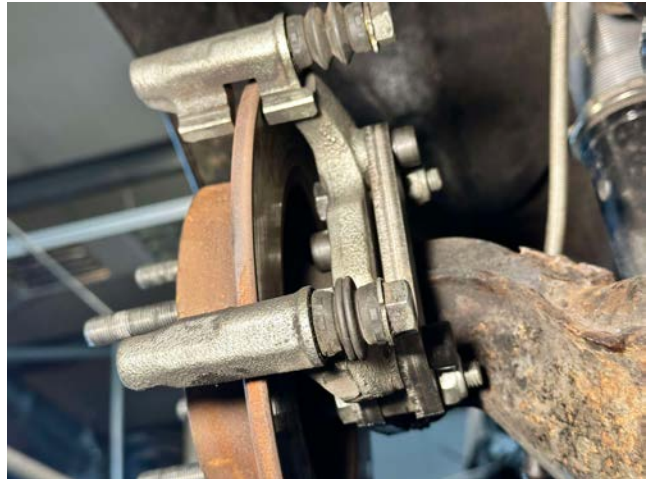
STEP 9 - INSTALL THE CALIPER IMPORTANT - THE CALIPER ARE HANDED (LEFT AND RIGHT) YOU NEED TO INSTALL THE LEFT CALIPER ON THE RIGHT SIDE, AND THE RIGHT CALIPER ON THE LEFT SIDE
